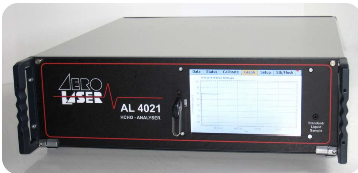
Fig. 2-1: AL4021 HCHO-analyzer. The inlet tube in the front is used for measuring liquid samples and supporting the liquid standard for calibration
