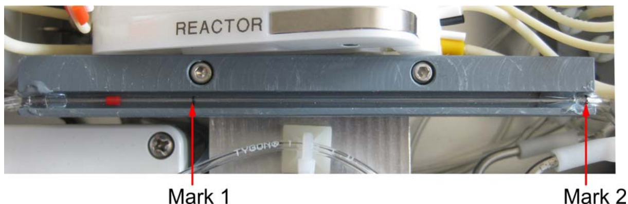
Fig. 5-29: Capillary for measuring the stripper speed. A bubble is produced to measure the time, which the solution needs to pass from mark 1 to mark 2. The volume between these marks is 200 \mu L. The time which the bubble needs is used for calculating the stripper speed.
